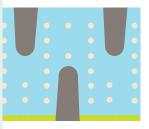
Ozone is bubbled into the water as a primary disinfectant to destroy bacteria and other microorganisms and improve taste.
